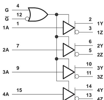
**SN65LVDS3487 logic diagram (positive logic)**
