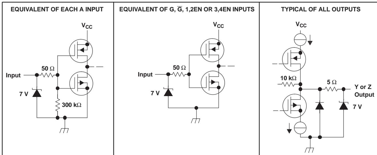
Figure 8. Equivalent Input and Output Schematic Diagrams
