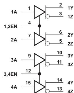
**SN65LVDS9638 logic diagram (positive logic)**
